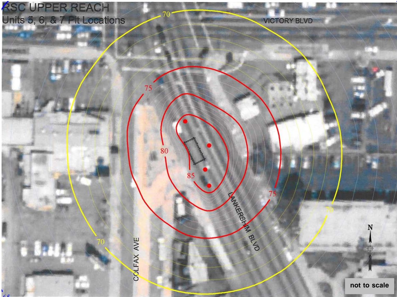
Figure 31: Jacking pit on Lankershim Blvd. south of Victory Blvd. (1-hr Leq)
