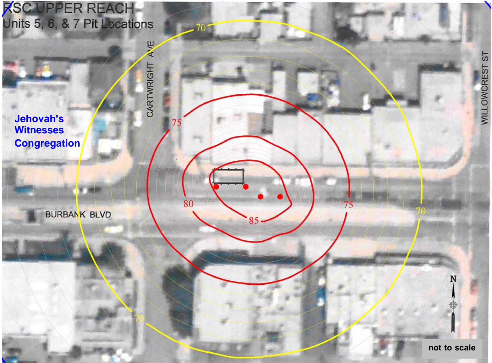
Figure 38: Jacking pit on Burbank Blvd. east of Cartwright Ave. (1-hr Leq)
