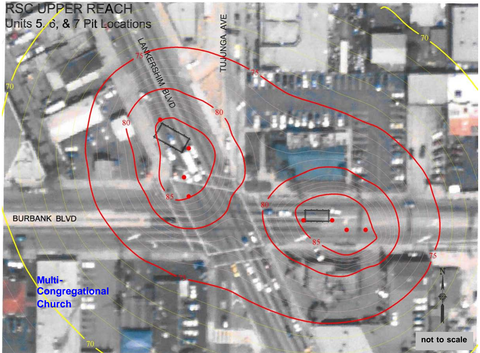
Figure 36: Jacking pits at intersection of Lankershim Blvd. and Burbank Blvd. (1-hr Leq)
