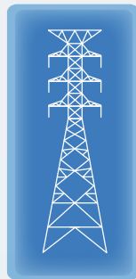
230 kV double-circuit structure
