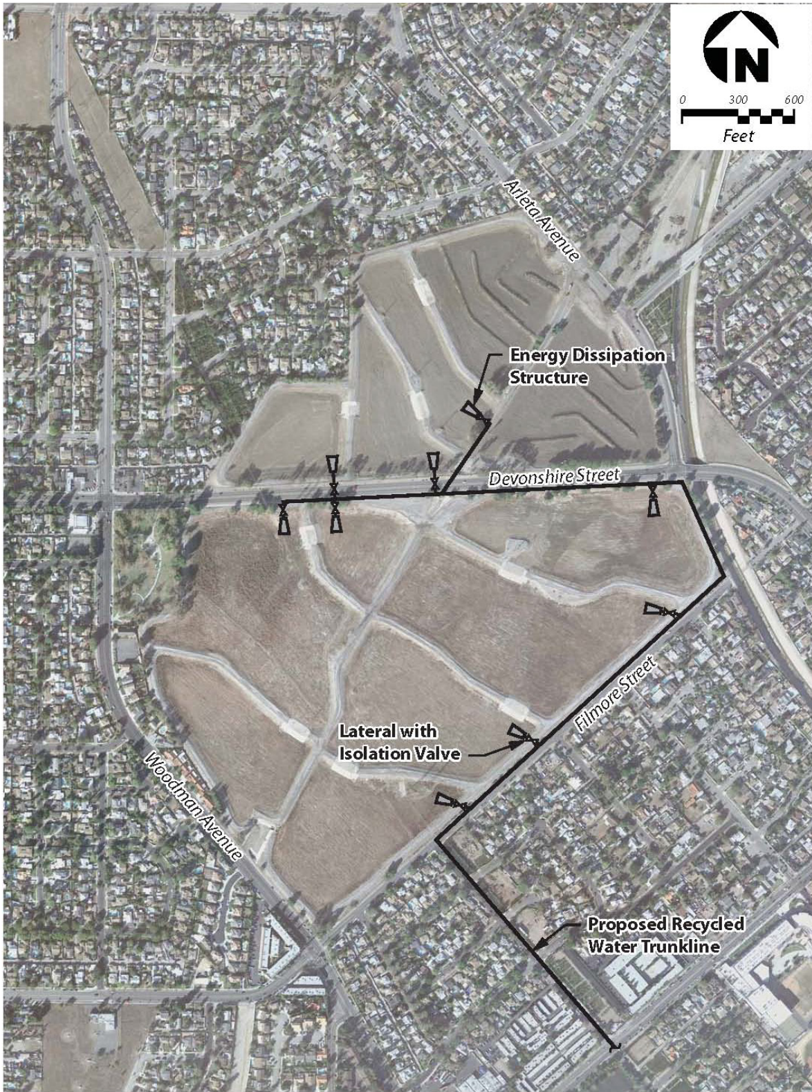
Figure 7-24: Proposed Facility Improvements at the PSG
