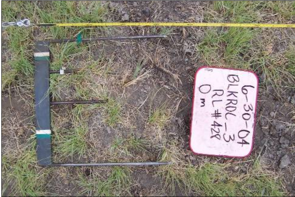
Figure 9.7 Example of a close-up view photo showing placement of the nested frequency frame.
