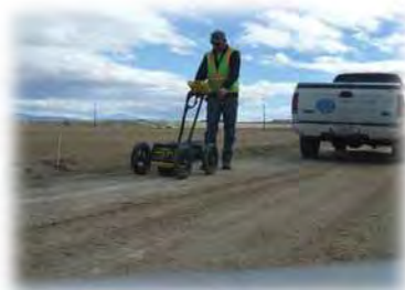
Data collection using the Noggin GPR (archive photo)
