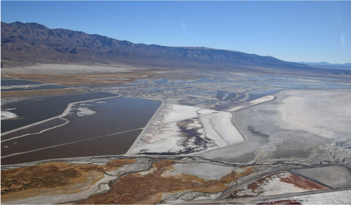
Figure 4-25. November 4, 2024, aerial image of DHA. Due to the high flows in 2023-24 RY, sediment was deposited at the southern end of the DHA. This deposition has shifted the channel to the west away from seasonal pond 15.
