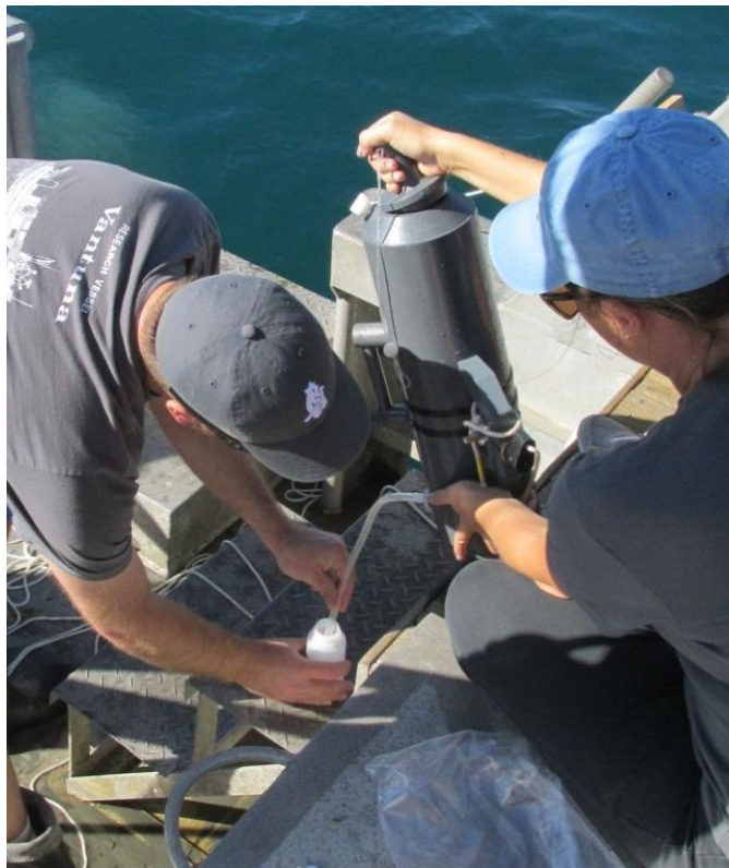
Figure 3-7: Niskin Water Sampler
