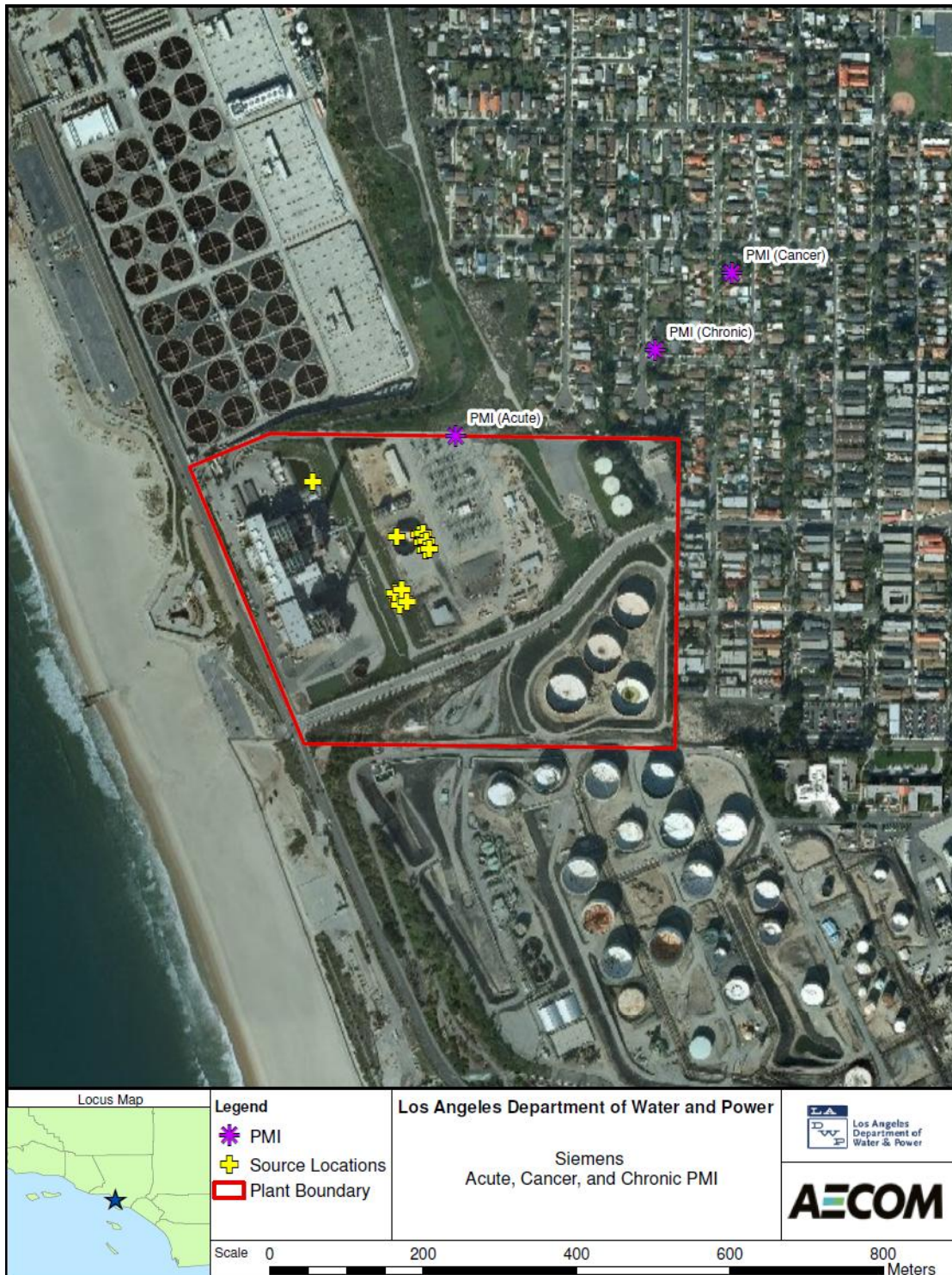
Figure 4 Point of Maximum Impact for Siemens Installation
