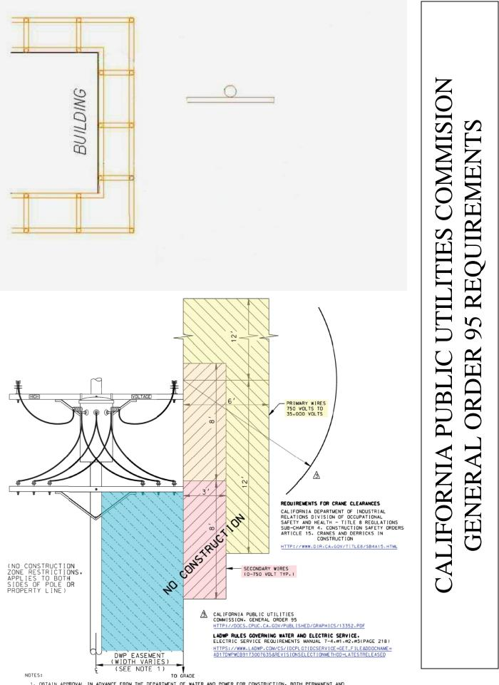
1. OBTAIN APPROVAL IN ADVANCE FROM THE DEPARTMENT OF WATER AND POWER FOR CONSTRUCTION. BOTH PERMANENT AND TEMPORARY. (I.E.SCAFFOLDING, CRANES, PATIOS, STRUCTURES, POOLS, SPAS, ETC.) WITHIN THE SHADED OR RADIAL CLEARANCE DESCRIBED ABOVE IN PROXIMITY TO POLES AND OVERHEAD WIRES.
