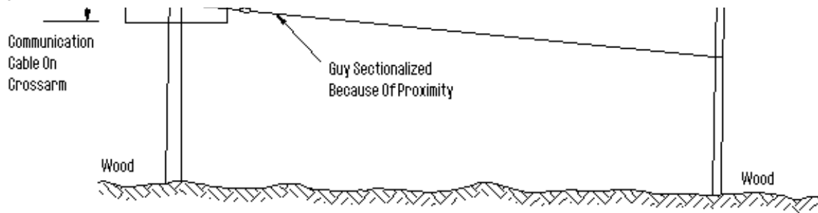
Figure 48 Sectionalization Of Overhead Guys On Jointly Used Poles
