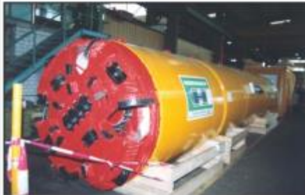
Microtunnel Boring Machine
